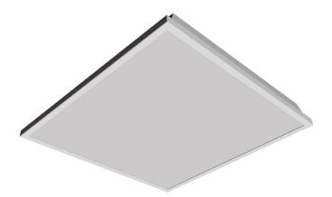
The Tegra LED panel is a bespoke modular luminaire designed to fit in to all SAS150 ceilings. The body is made from powder coated steel giving a screwless appearance from under the ceiling. The diffuser is made from high efficiency PMMA which gives the luminaire optimum performance.
